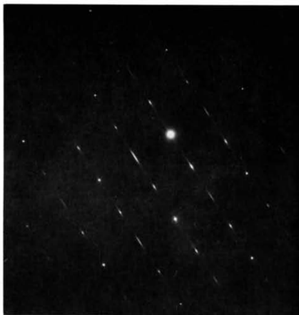
Fig. 1. Electron diffraction pattern from a thin crystal of magnesium fluorogermanate, taken with the beam parallel to the a axis, showing the streaks parallel to the c^* axis. (Courtesy of Dr Peter Kunzmann.)
